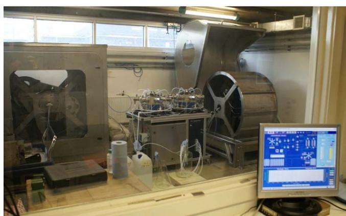
**Figure 1:** Prototype 4.6 litre DE-Maxi centrifuge on the left and the newly installed 18 litre DE-MAXI centrifuge on the right. In the centre and on the screen in the control room in the foreground are the liquid handling system and control software
